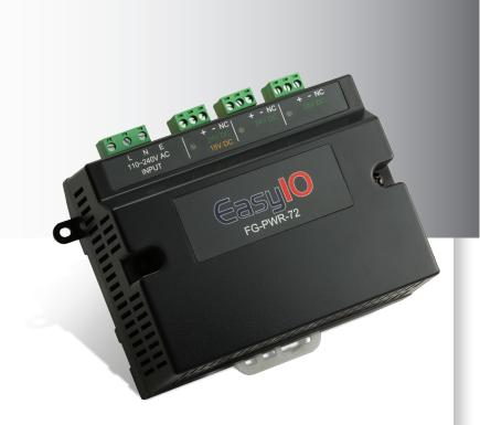
A High quality DIN Rail Mounted isolated 3  $\times$  24VDC, 1 amp each, BMS Power Supply. The first output can also provide 15V DC using a jumper setting.
